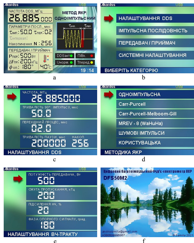
Fig. 7. Graphical interface of the control system of the radio spectrometer: a – user interface screen, b – menu entry, c – synthesizer settings, d – choice of technique, e – setup the RF path, f – dynamic screen saver.
