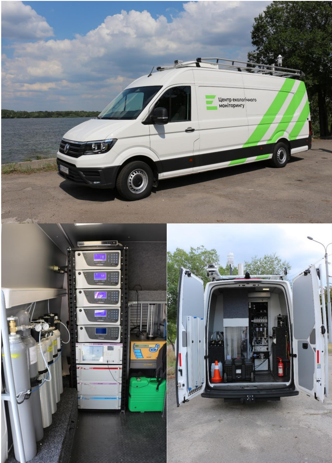
Fig. 3. General view of the reference mobile environmental monitoring station and the system of instruments of the station
