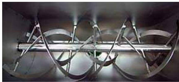
Figure 4. shaft with two tapes of a design like "S"
