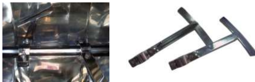
Figure 2. shaft and working bodies of the conical mixer.
