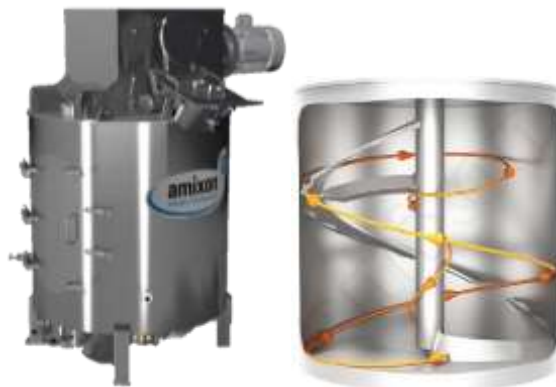
Figure 5. vertical single-shaft belt mixer and product circulation scheme
