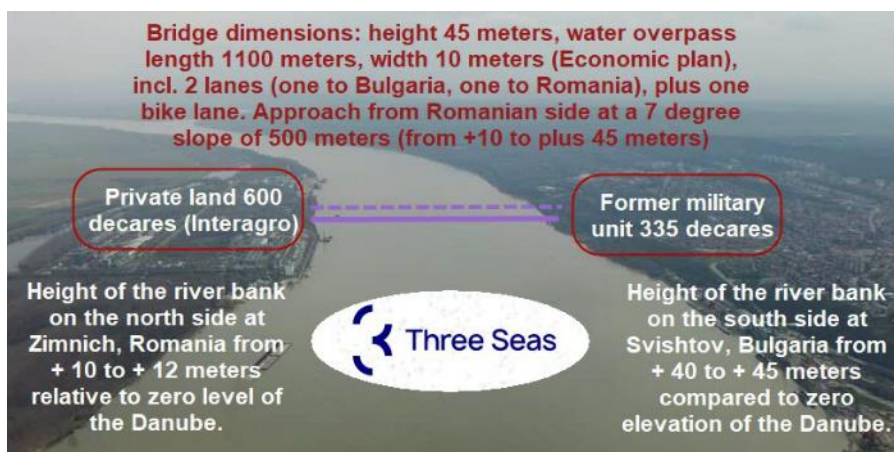
Figure 1. Location and dimensions of the Bridge Danube South: Svishtov – Zimnicea
