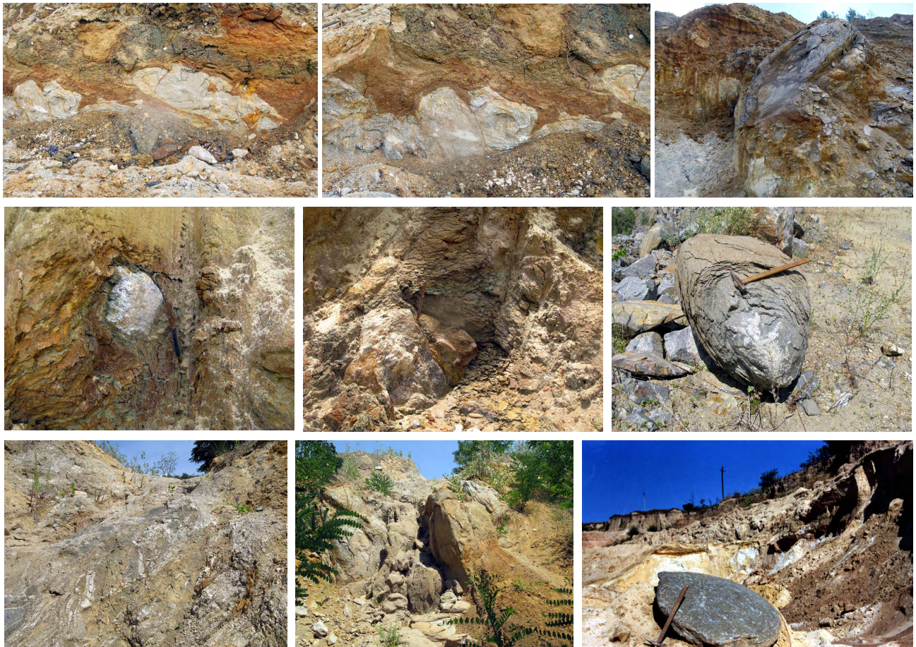
Fig. 11. Consequences of physical-chemical weathering of crystalline rocks of the Precambrian basement in the form of disintegration, ferruginization, hydration reaction, dialysis, hydrolysis and desquamation
