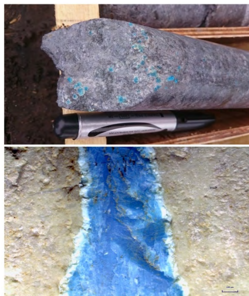
Fig. 8. Turquoise ( \text{CuAl}_6(\text{PO}_4)_4(\text{OH})_8 \cdot 4\text{H}_2\text{O} ) mineralization in the Reza gold deposit: turquoise minerals observed on fractures, rhyodacite core piece (the upper); turquoise mineral fragment in rhyodacite rock, photos taken under Leica S8AP0 Binoculars (the following).
