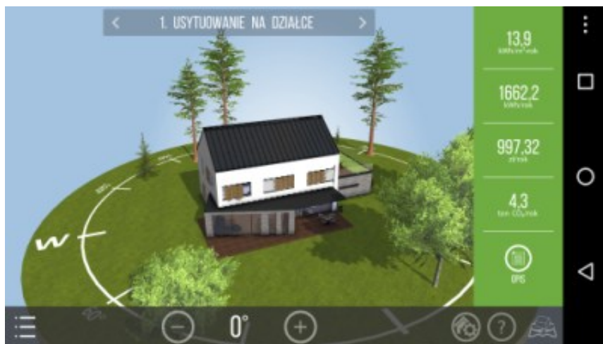
Figure 8.3. The screen indicating the possibility of rotation of the building relative to the cardinal directions [19]
