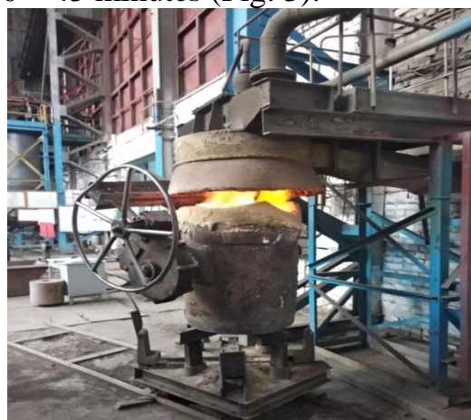
Figure 3. In the process of heating the bucket on a gas stove
