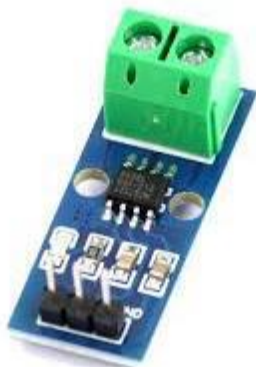
Figure 6: ACS712 current sensor, Hall Effect.
