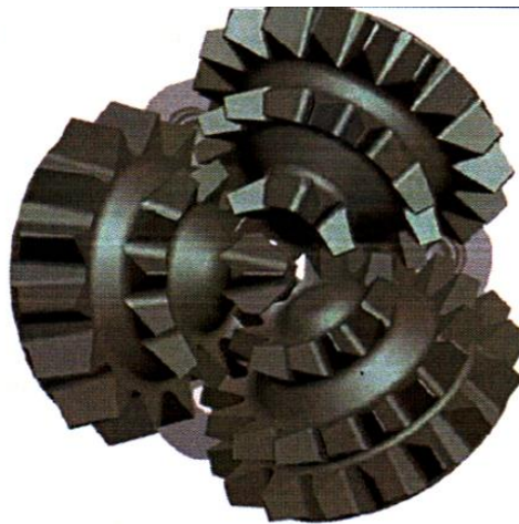
Figure 1. Roller-bit 295,3 SB IADC code 217
