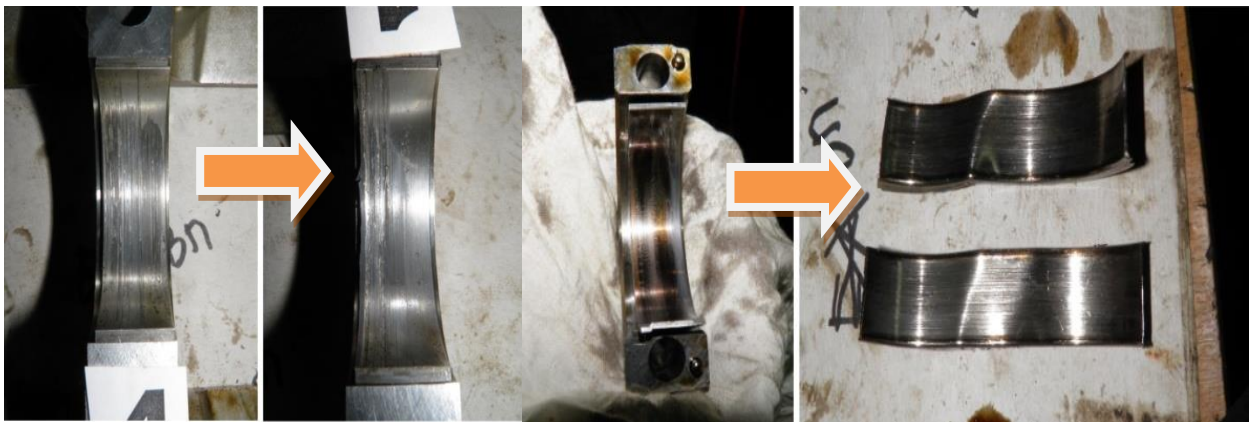
Fig. 3. Damage to all bearings, both main (left) and connecting rod ones (center and right)
