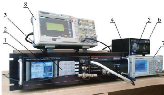
Fig. 4.2 Measurement setup for the observation of NQR: 1 – portable digital multipulse NQR spectrometer, 2 – graphical display, 3 – settings panel, 4 – NQR signal sensor, 5 – tuning capacitor, 6 – probe coil, 7 – signal generator, 8 – oscilloscope
