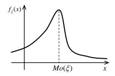
It is customary to denote the mode of distribution of a random variable  $\xi$  by  $Mo(\xi)$ . A distribution with a single mode is called **unimodal** (for example, a normal distribution), in the opposite case – **polymodal** (for example, a uniform distribution on a segment).
