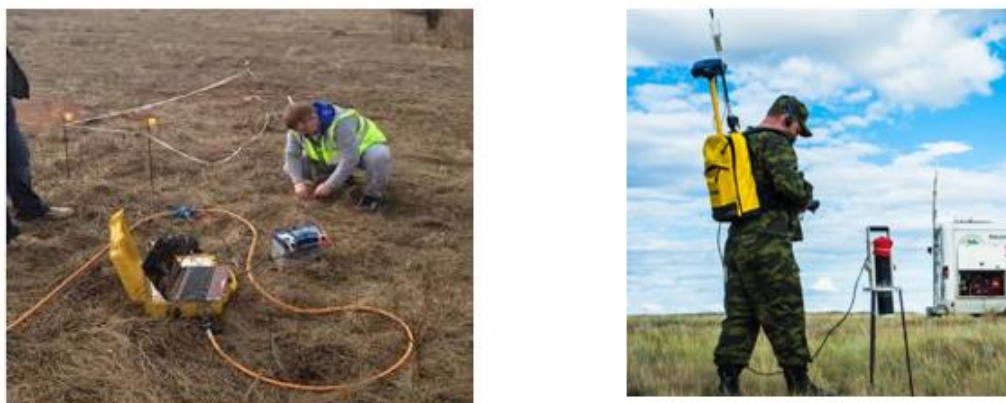
Fig. 1 - Seismic survey (a) and coordinates determination of boreholes by GPS receivers (b).
