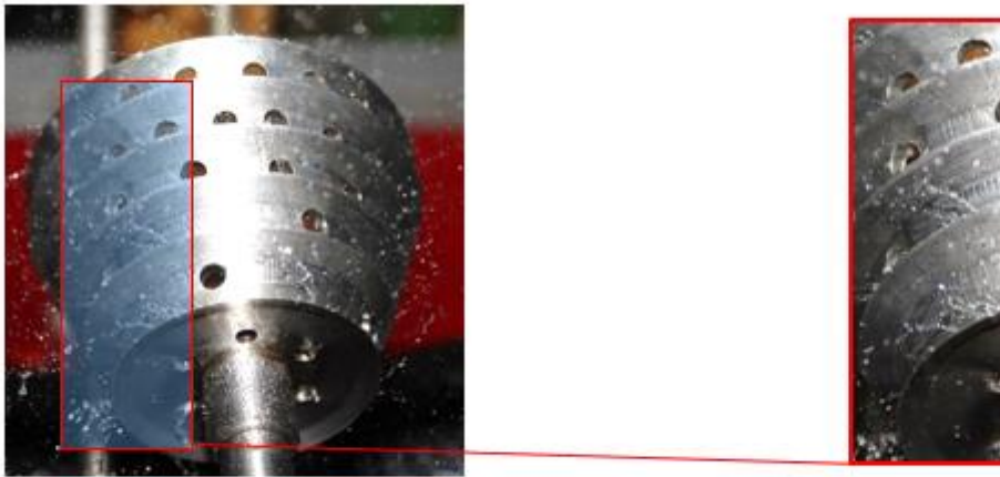
Figure 4 - Photo of the outer surface of the rotary dispersant in the distribution of the model fluid, at \Gamma_v = 3,71 \cdot 10^{-4} \frac{m^3}{m^2 s} , \omega = 439 1/s
