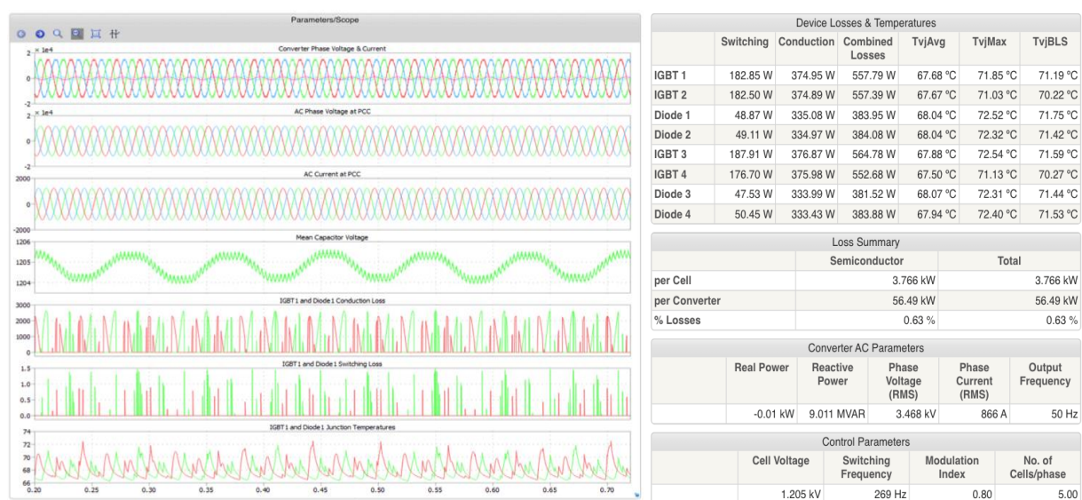
Fig. 5. Calculation curves (left) and calculated parameters for the RPCS variant with the lowest loss when using a HiPak IGBT module
