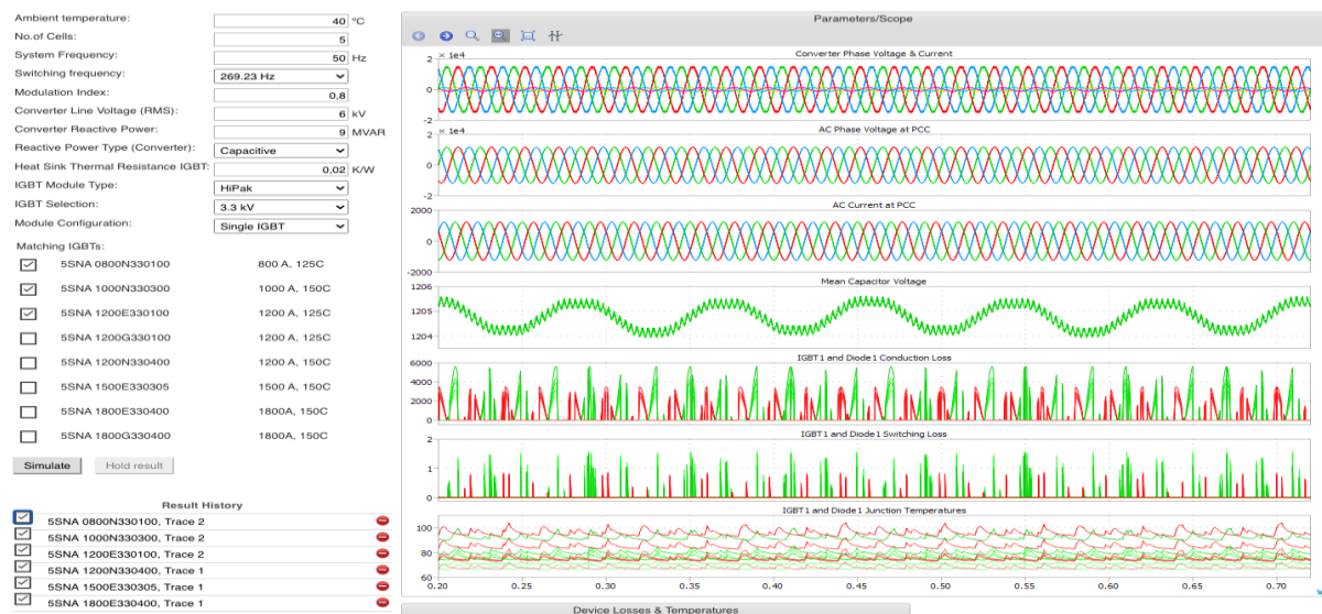
Fig. 2. Calculation results for the specified 6 variants of IGBT modules
