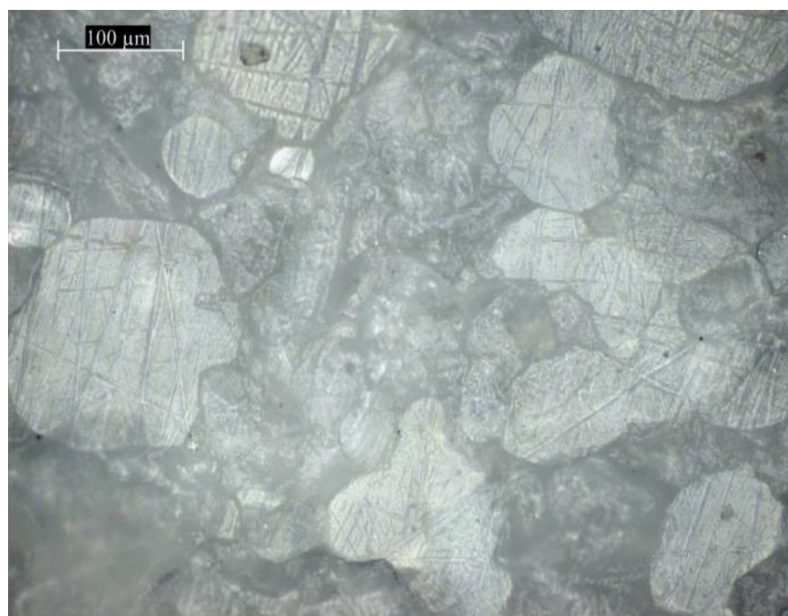
Figure. 3. Microphotographs of modified PTFE specimens obtained a) by cold pressing, by sintering at a temperature of T = 3930C , b) after sintering, which stood under the press for 24 hours.
