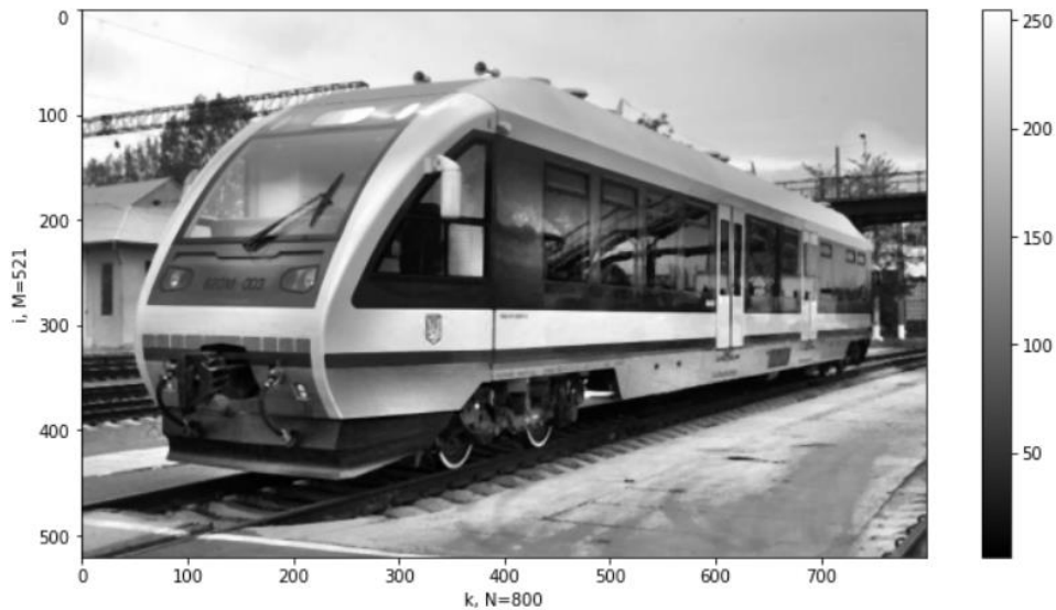
Fig. 7 – The image f_C with the removed inhomogeneous background and the increased local contrast received on the basis of the initial image f (fig. 1); window dimensions M_w = N_w = 64 (with filtration of envelopes)
