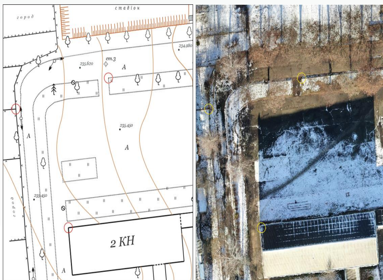
Fig. 15. Comparison of aerial photography results: a – topographic plan; b – orthophoto plan
