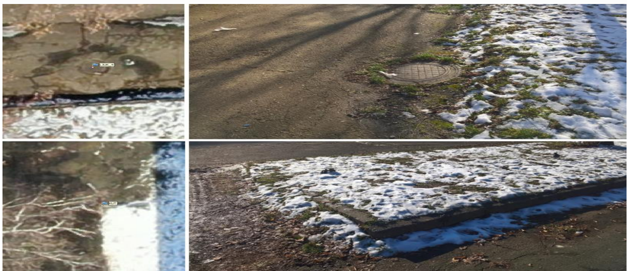
Fig. 5. Look of objects chosen as points of GCP (ground control points) on the territory of school #6: a – marking of the sewer hatch and its appearance on the ground; b – border marking and its appearance on the ground
