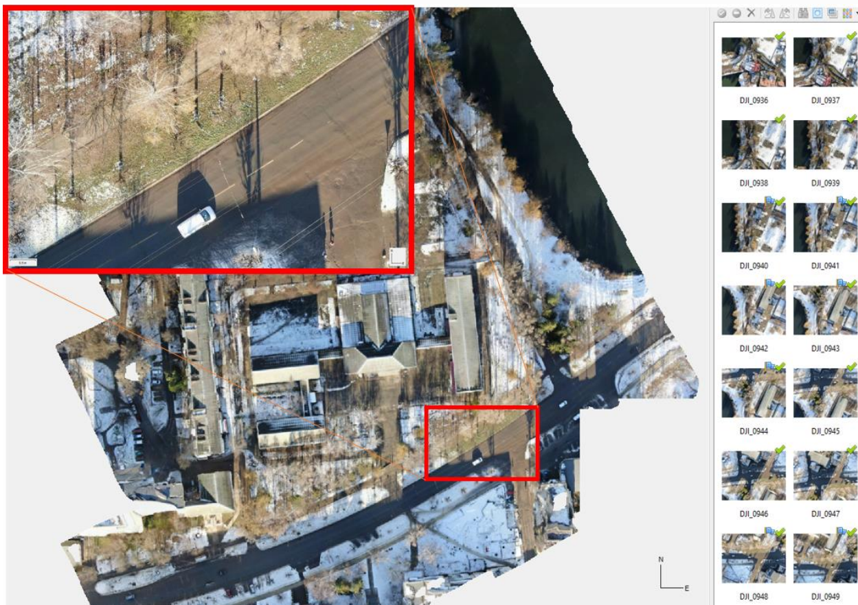
Fig. 14. View of the created orthophoto plan
